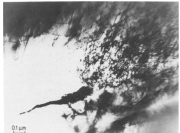
Figure 7 Dislocation substructure formed ahead of the crack tip in a foil of niobium-10 at % vanadium alloy deformed in situ in the tensile stage. The crack is subject to a shear stress parallel to the crack faces. Multiple g vectors are operating.
