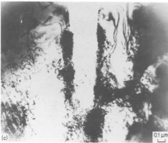
Figure 5 (a) Crack nucleation in a region of high dislocation density observed close to the edge of the foil of niobium-10 at % vanadium alloy deformed in situ in the tensile stage of the microscope. Multiple g vectors are operating. (b) A well defined tensile crack with surrounding dislocation substructure formed after further deformation of the foil of niobium-10 at % vanadium alloy in situ in the tensile stage. Multiple g vectors are operating. (c) Crack growth with surrounding dislocation substructure observed after further deformation of the foil of niobium-10 at % vanadium alloy in situ in the tensile stage. Multiple g vectors are operating. (d) Crack tip blunting due to extensive deformation and formation of dislocation substructure surrounding the crack in the foil of niobium-10 at % vanadium alloy deformed in situ in the tensile stage. Multiple g vectors are operating.
