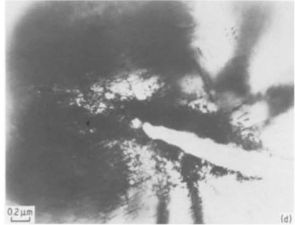
Figure 8 (a) Formation of dislocation substructure, slip traces and ledge steps responsible for continuous plastic crack growth in the foil of niobium–10 at % vanadium alloy with hydrogen deformed in situ in the tensile stage of the microscope. Multiple g vectors are operating. (b) Further development of substructure at the crack tip as a result of crack growth in the foil of niobium–10 at % vanadium alloy with hydrogen deformed in situ in the tensile stage. Multiple g vectors are operating. (c) Extensive dislocation multiplication in line with the crack observed after further crack growth in the foil of niobium–10 at % vanadium alloy with hydrogen deformed in situ in the tensile stage. Partial thinning of a region immediately ahead of the crack is also observed. Multiple g vectors are operating. (d) Void formation and growth observed ahead of the crack tip after further crack growth in the foil of niobium–10 at % vanadium alloy with hydrogen deformed in situ in the tensile stage. Multiple g vectors are operating. (e) Void coalescence and dislocation substructure observed ahead of the crack tip in the foil of niobium–10 at % vanadium alloy with hydrogen after further deformation in situ in the tensile stage. Multiple g vectors are operating.
